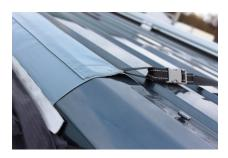
WARNING: Never unzip the zips on the protective sleeves whilst the AirFrame Tubes are inflated. This will result in the tube bursting or ballooning out of the sleeve causing damage to the tube and the sleeve. This is not covered under the warranty.
